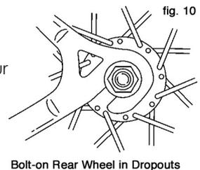
**Bolt-on Rear Wheel in Dropouts**
