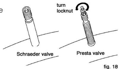
up the valve. The adapter fits into the Schraeder pump fitting. Close the valve after inflation. To let air out of a Presta valve, open up the valve stem lock nut and depress the valve stem.
